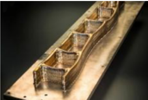
Typical titanium part produced by high deposition rate AM
